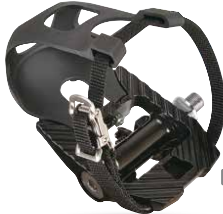
SIDE A : Platform + Toe clip attachable.
