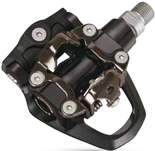
SIDE B: EPS-M (Compatible with Shimano SPD).
