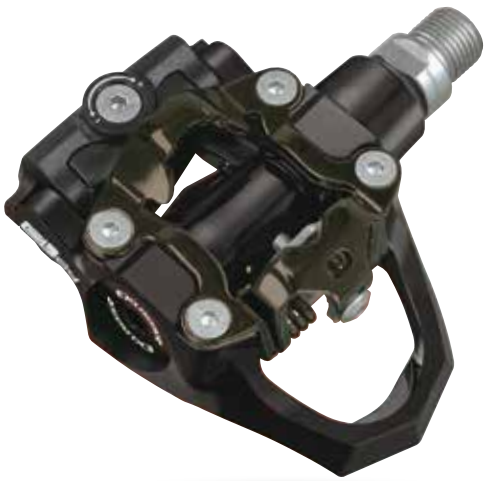
SIDE B: EPS-M (Compatible with Shimano SPD).
